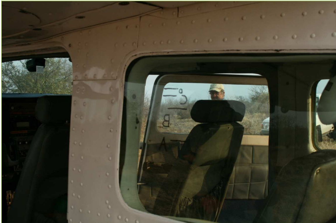
Figure 2: Marks on aircraft window to assist with range.
